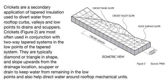
When designing a cricket, two items need to be designed – slope and configuration of the cricket. A general rule for designing sufficient slope in crickets is that its slope shall be twice the slope of the adjacent roof field. Typically, that will keep water from remaining on the cricket surface. Some residual water could be expected but it should dissipate within 48 hours.<sup>3</sup>
